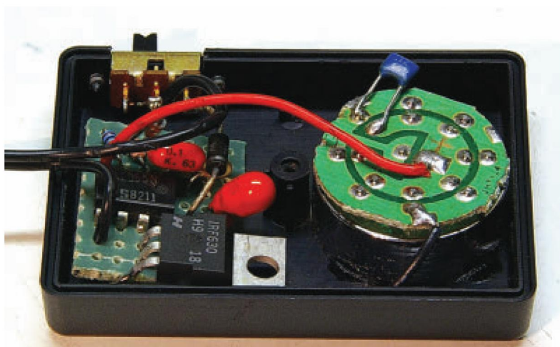
■ PHOTO 5. Through-hole circuitry inside the task light.
